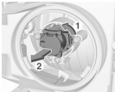
1. Rotate cap anticlockwise and remove it.
