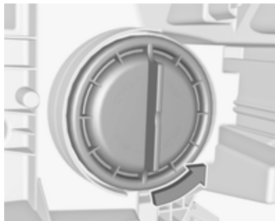
1. Rotate cap anticlockwise and remove it.
